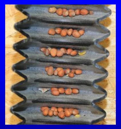
Accordion type drop tubes hold and dump seed.
