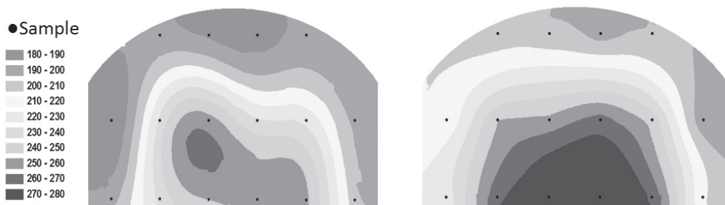
Figure 2 Crop density [kg DM m -3 ] of maize across the silo face LD 7% film extension (left) and HD 9.5% film extension (right).
