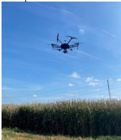
Figure 2: Demonstration of capturing image data over a corn field with a RedEdge camera drone.
