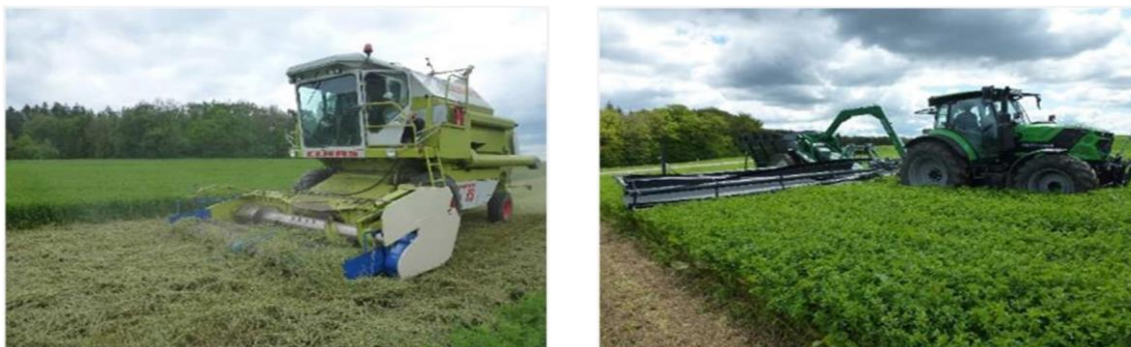
Figure 1: Adapted combine harvester for harvest of alfalfa leaves (left); Top Cut Collect machine for harvest of alfalfa tops (right). (© J.Maxa)
